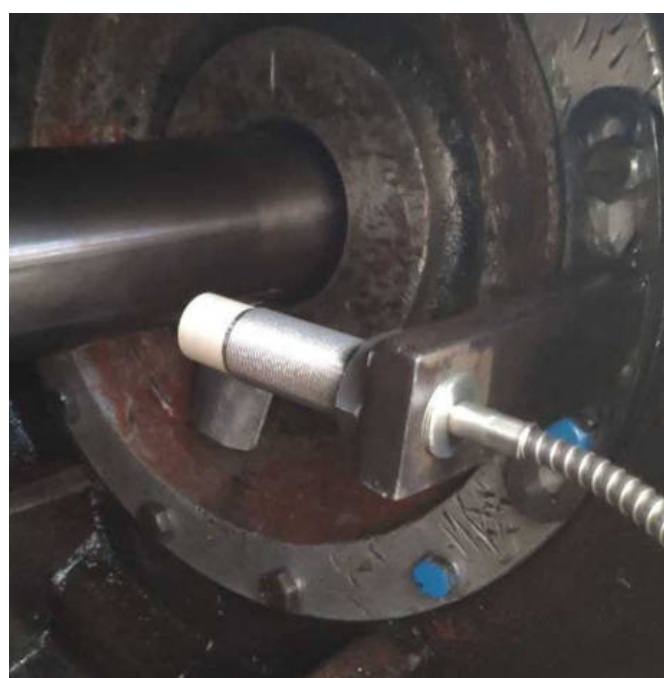
Eddy-current sensors of RPE «TIK» on pump units
