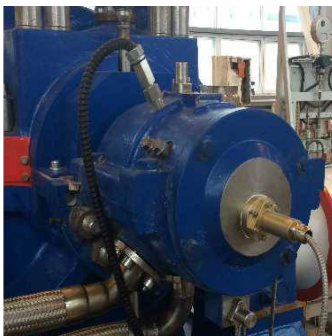
Eddy-current sensors of RPE «TIK» on pump units
